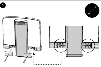
**4.** Raise the seat to remove the bracket covers to get to the mounting holes. Using a level and a pen, mark the hole positions, making sure that the seat is horizontal.
