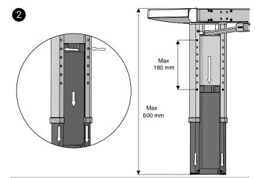
**2.** Adjust the leg height by pushing in the leg pins and slide the adjustable leg downwards. Always ensure that the leg pins are locked into position and the leg height cannot move before the user sits down.
