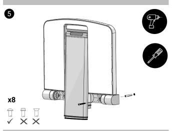
**5.** Drill the holes and insert the appropriate fittings. (Fittings not supplied) Do not use countersunk heads or over-tighten the screws.
