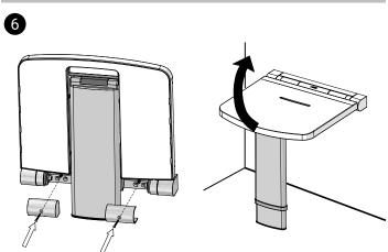
**6.** Position the seat over the holes and insert appropriate fittings and secure in place. Replace the bracket covers and test the seat operation.
